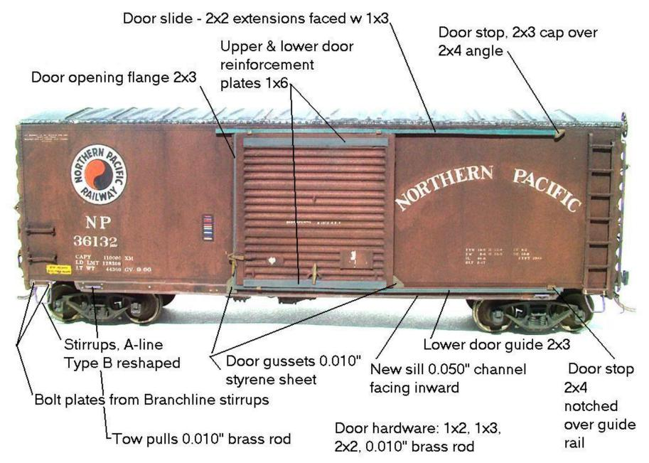
Photo 3: HO scale model with major car side detail modifications highlighted and labeled. (C. Frissell photo).
